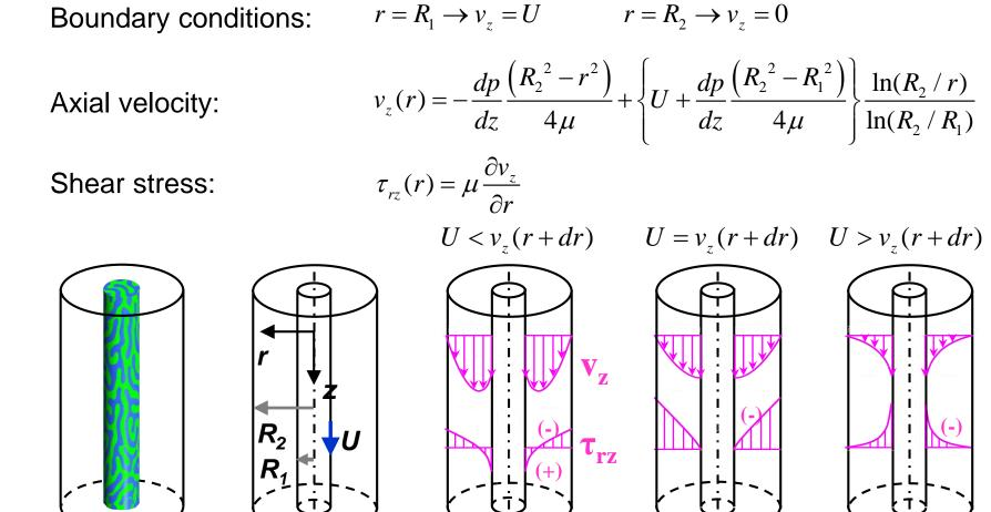
The fiber can either move slower, at equal speed or faster than the water.
