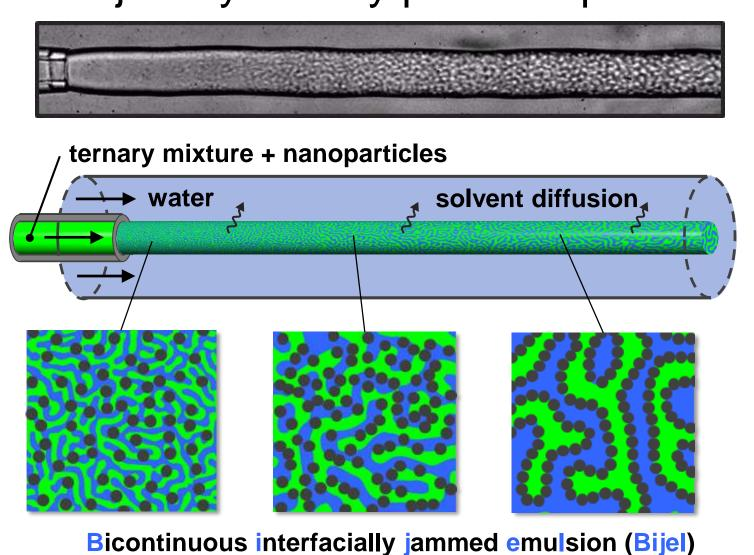
A liquid mixture with nanoparticles is extruded into a water flow
