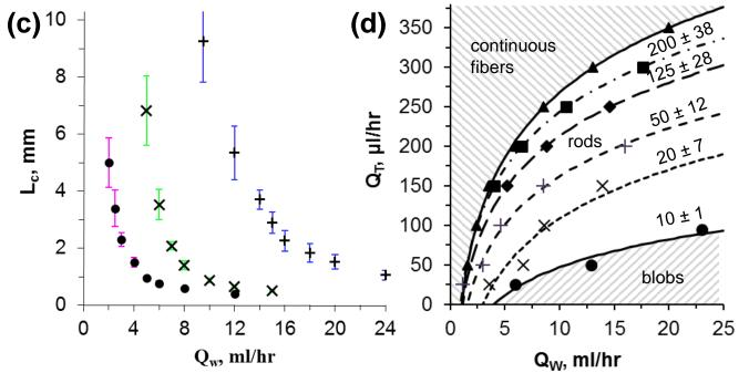
In (c) we plot the fiber-segment length  $L_{\rm C}$  for constant flow rates of the liquid mixture  $(Q_T)$  vs. the water flow rate (Q<sub>w</sub>). A complex relationship for the fiber aspect ratio as shown in (d) is found.
