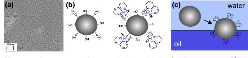
We use silica nanoparticles as building blocks for the capsules (SEM) image in (a)). Silica is naturally hydrophilic but can become partially hydrophobic upon surface modification. We alter the hydrophobicity of silica by the adsorption of positively charged 8HQ on the negatively charged silica particles (b). After this modification the particles attach
