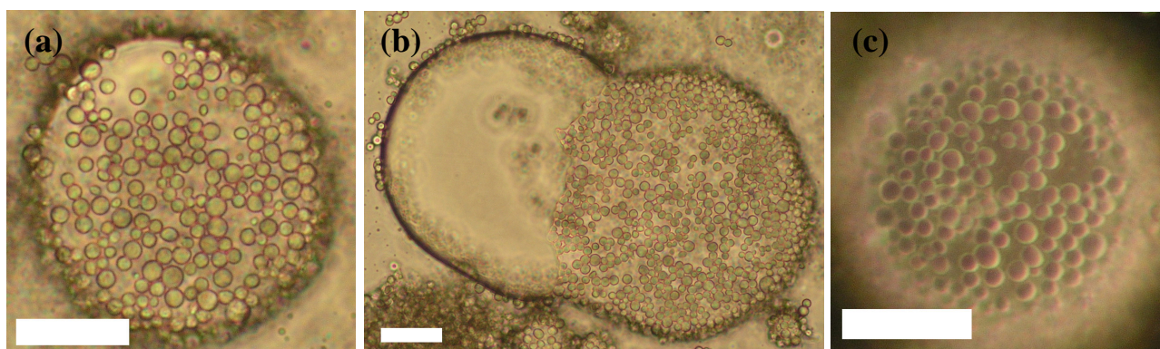
Figure 35. PE-ML coated PSE-droplets attached to DEP droplets. (b) two droplets were probably coated during coalescence, the left side of the droplet is attached to the 8-HQ hydrophobized microscopic glass coverslip (c) dark field micrograph of a droplet. Scale bar always 20 \mu m
