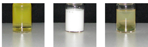
Figure 33. Destabilization of a stable emulsion by either adding acid or base
